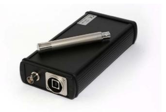
Simply connect the USB interface to one USB port and connect the interface to the microphone.
