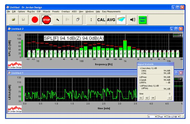
The SPL meter should display 94dB. It is important that you see a peak at 1kHz. The A and Z weighted level should have a deviation of max 0.3dB. A small mismatch between the two
