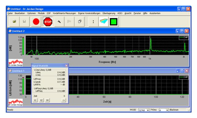
The default frequency resolution is 1.3Hz. You can increase the frequency resolution by adjusting the FFT size. However, the higher is the frequency resolution, the lower the time resolution. The system will "move slowly".
