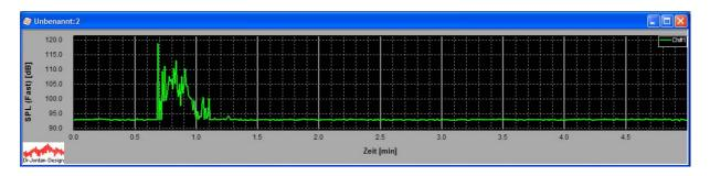
With the following section you can plot the narrow band SPL with a center frequency of 1000Hz.
